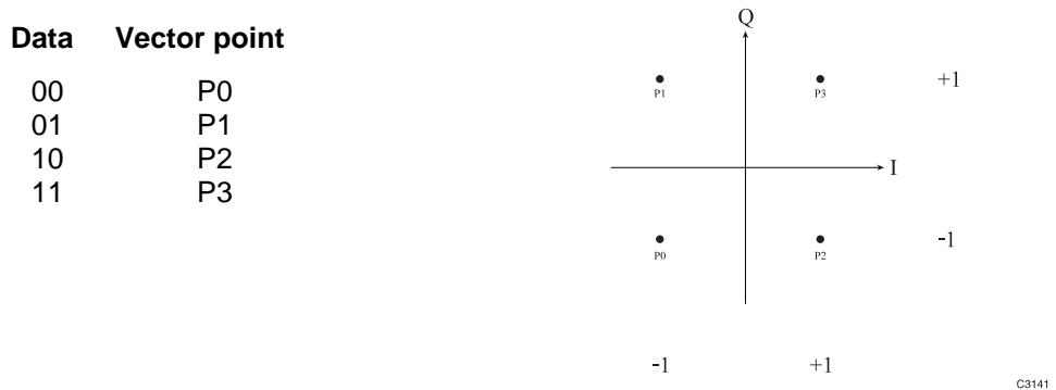
Fig. 3-33 Time offset QPSK constellation
