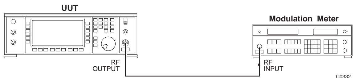
Fig. A-28 Accuracy of SDM signal path test set-up
